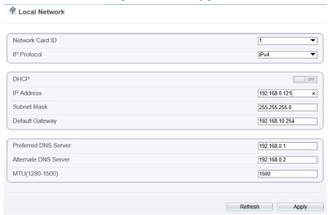
Step 2 Set the parameters according to Table 4-2.
